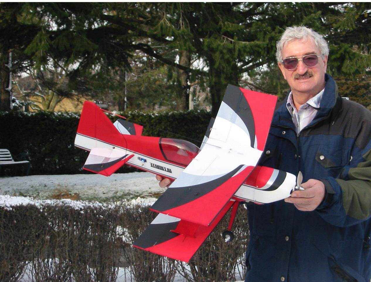
more precise maneuvers with its interlocking wing design and carbon fiber stiffeners and blade spars. The ULTIMATE FX can handle more WIND THAN MOST FOAMIES. It weighs 14oz – ready to fly. You can buy this airplane from Pinnacle Hobbies (Markham)
